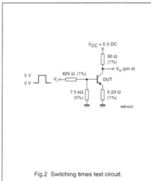
Fig.2 Switching times test circuit.
